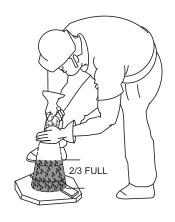
Figure 35-B. Slump Test (2/3 Full)
